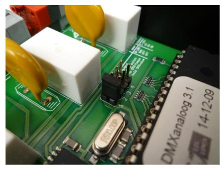
In the picture above, jumper 1 is closed and jumper 2-3-4 are in open position.
