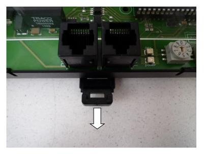
If the product is used in a situation where heavy mechanical shocks can be expected, we advise to remove the plastic din-rail enclosure and bolt the analogue converter PCB directly on a metal base. Use bolts and nuts M3 to attach the PCB. Use proper spacers to avoid electrical contact between solder pads and the metal parts of the housing.
