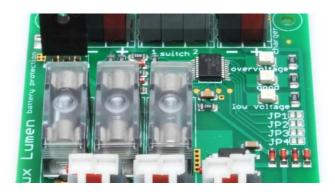
Only replace the fuse with the same type and current installed in the battery protection board.
