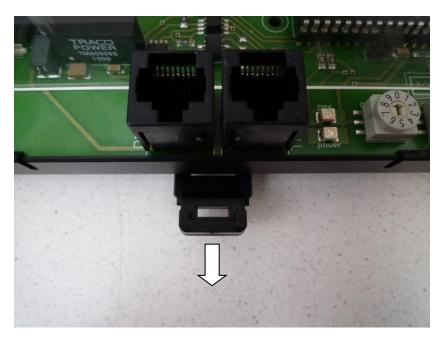
If the product is used in a situation where heavy mechanical shocks can be expected, we advise to remove the plastic din-rail enclosure and bolt the relay card PCB directly on a metal base. Use bolts and nuts M3 to attach the PCB. Use proper spacers to avoid electrical contact between solder pads and the metal parts of the housing.
