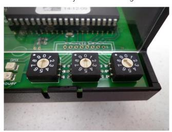
*Note*: If the card is oriented that the text on the PCB is readable, the positions of the wheels will affect following address-setting:
