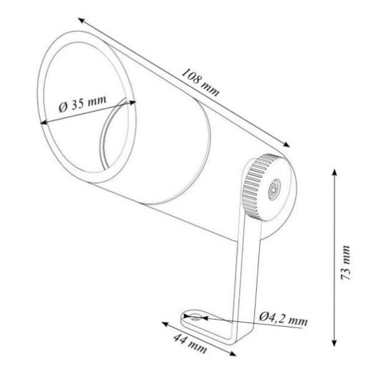
The dimensions of the main housing, a cylindrical aluminum lathed part, is  $\phi$ 35mm with 108 mm length (snoot included).
