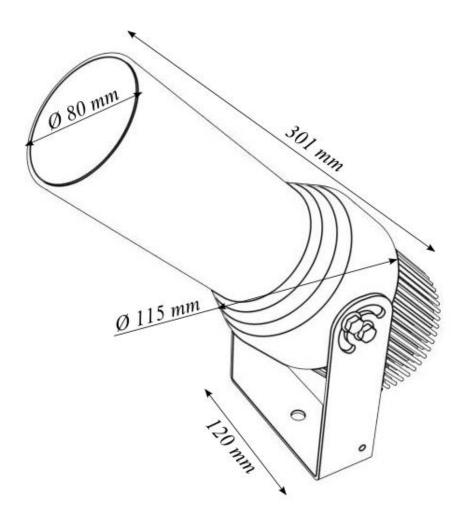
The height with bracket is max. 178 mm.
