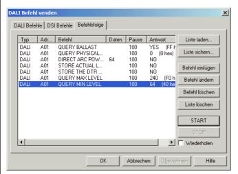
Use the tab "command list (Befehlsfolge)" to create and save command sequences, which will be used frequently. A command list may be helpful for initial initialization of the interface: set and store values for min level, max level etc.
