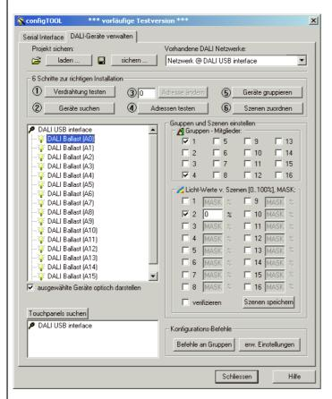
We recommend to use our USB-DALI Adapter for a simple setup of the DALI system. This chapter shows a quick introduction to DALI programming using our interface. If using other type of DALI controllers, please refer to the respective instruction manual.
