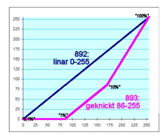
programming address: 892: linear characteristic 000...255 (DEFAULT) programming address: 893: bended characteristic 086...255
